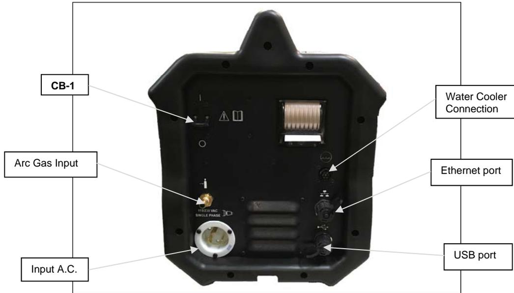
2. Connect Argon (or mixed gas) from an external source to the Model 217P **ARC GAS INPUT** connector, **the ARC GAS is monitored by the computer and MUST be run through the power supply to avoid a FAULT**. Connect the weld head electrode, ground, motor control, and gas line via the 24 inch cheaters or 15-foot adapter cable to the power supply.
