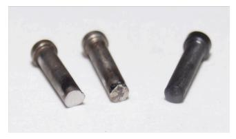
In addition to wear of the home pin causing frequent adjustments/replacement, standard home pins are prone to damage. A damaged pin (burrs, wire-edge, etc.) can 'stick' in the bushing, causing homing failures. The CSI home pin is more durable and forgiving, even after 10,000+ cycles.
