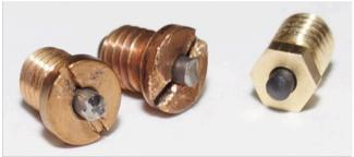
The flat-blade slot in standard home pin bushings provide less support for the home pin. This allows the home pin to flex and wear unevenly. Hex head design gives consistent home pin support, inimizing pin damage.
