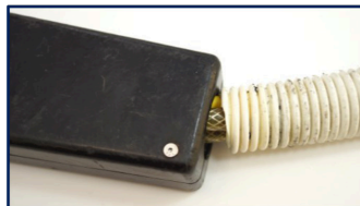
Cable Sheath can tear away from the handle in standard assembly causing wire & cable damage.
