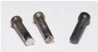
Home pin is made from non-conductive material
